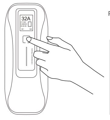
Press the button and switch charging current (Only for current-switchable version)
