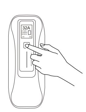
Press the button and switch charging current The process in Figure 2 must be performed before Figure 3
