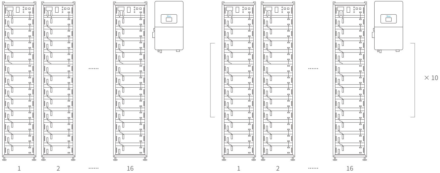
Maximum support for 16 racks of batteries in parallel
