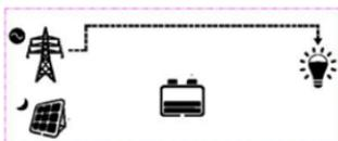
The battery voltage goes lower than or equal to AON. Simultaneously, it has not been charged to AOF. Instead, the utility supplies the load and charges the battery.
