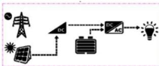
When the battery voltage goes lower than or equal to the LVD point, the utility supplies the load, and PV charges the battery.
