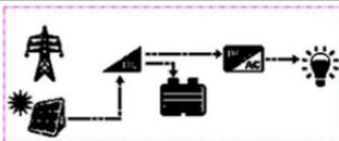
When PV power is lower than or equal to load power, PV stops charging the battery. Instead, it supplies the load together with the battery.
