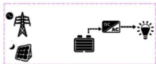
The battery voltage goes lower than or equal to AON. Simultaneously, it has not been charged to AOF. Instead, the utility supplies the load and charges the battery.
