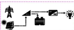
When PV power is lower than or equal to load power, PV stops charging the battery. Instead, it supplies the load together with the battery.
