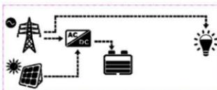
When PV power is higher than  $MCC \cdot V_{BAT}$ , the PV charges the battery alone and supplies the load together with the utility.
