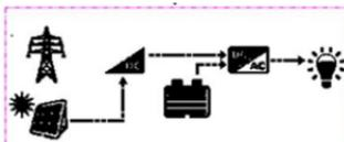
When the battery voltage goes lower than or equal to the LVD point, only PV charges the battery.
