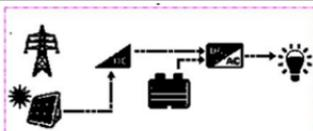
When the battery voltage goes lower than or equal to the LVD point, only PV charges the battery.
