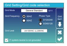
Grid Setting/Connect Normal connect Normal Ramp rate 10s Low frequency 48.00Hz High frequency 51.50Hz Grid Set2 265.0V Low voltage 185.0V High voltage Reconnect after trip Reconnect Ramp rate 36s Low frequency 48.20Hz High frequency 51.30Hz 187.0V High voltage 263.0V 1.000
