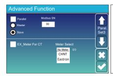
**Ex\_Meter For CT:** when using zero-export to CT mode, the hybrid inverter can select EX\_Meter For CT function and use the different meters.e.g.CHNT and Eastron.
