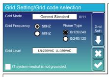
Grid Mode:General Standard、UL1741 & IEEE1547、CPUC RULE21、SRD-UL-1741、CEI 0-21、Australia A、Australia B、Australia C、EN50549\_CZ-PPDS(>16A)、NewZealand、VDE4105、OVE-Directive R25. Please follow the local grid code and then choose the corresponding grid standard.
