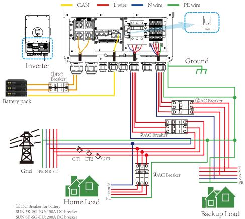
① DC Breaker for battery SUN 5K-SG-EU: 150A DC breaker SUN 6K-SG-EU: 200A DC breaker SUN 8K-SG-EU: 250A DC breaker SUN 10K-SG-EU: 300A DC breaker SUN 12K-SG-EU: 300A DC breaker
