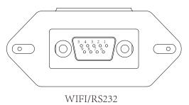
This RS232 port is used to connect the wifi datalogger
