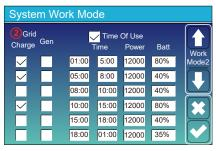
Time of use: it is used to program when to use grid or generator to charge the battery, and when to discharge the battery to power the load. Only tick "Time Of Use" then the follow items (Grid, charge, time, power etc.) will take effect.
