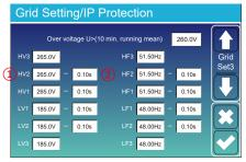
HV1: Level 1 overvoltage protection point;
