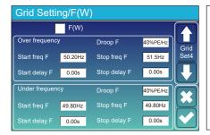
**FW**: this series inverter is able to adjust inverter output power according to grid frequency.
