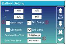
(2) This is Grid Charge, you need select. Start =30%: No use, Just for customization. = 37A: It indicates the Current that the Α Grid charges the Battery. Grid Charge: It indicates that the grid charges the battery.
