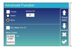
**Ex\_Meter For CT:** when using zero-export to CT mode, the hybrid inverter can select EX\_Meter For CT function and use the different meters.e.g.CHNT and Eastron.
