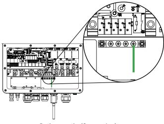
Earth connection(Copper wires)
